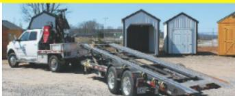
Building will arrive fully constructed at the customers site on a truck and trailer similar to the picture. Our delivery crew will level the building with blocks provided by the customer. If the customer has a tight spot we have a machine called a "mule", used for moving the building through the customers yard without the additional bulk and size of the truck when access is limited.
